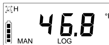
Fig 4: EVt showing reading in high alarm while logging.
